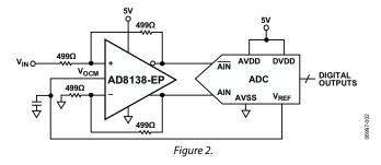
The AD8138-EP's differential output helps balance the input to the differential ADCs, maximizing the performance of the ADC.
